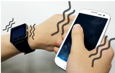
Figure 1. Vi-Bros is a new interface that simultaneously utilizes two mobile devices, a smartphone and a smartwatch, to provide users with intuitive guidance during indoor navigation. A smartphone vibrates when users have to turn right at an intersection. A smartwatch vibrates when users have to turn left at an intersection.
